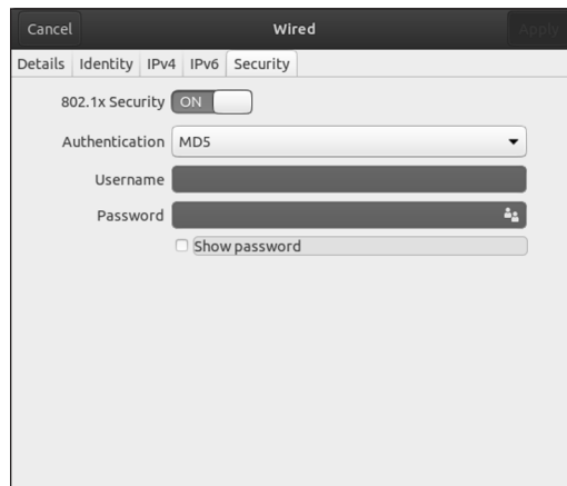
FIGURE 2-4: The Security tab allows you to configure the strength of your authentication.
